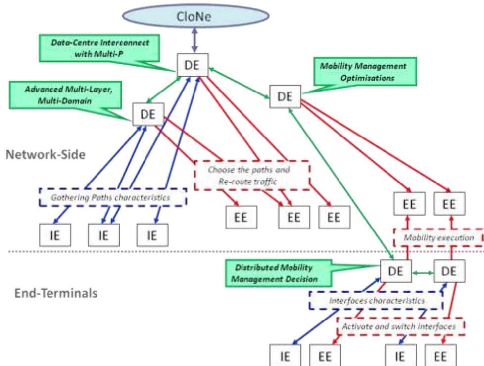
Figure V: Mobile Access and Data-Centre Interconnection use-case.
